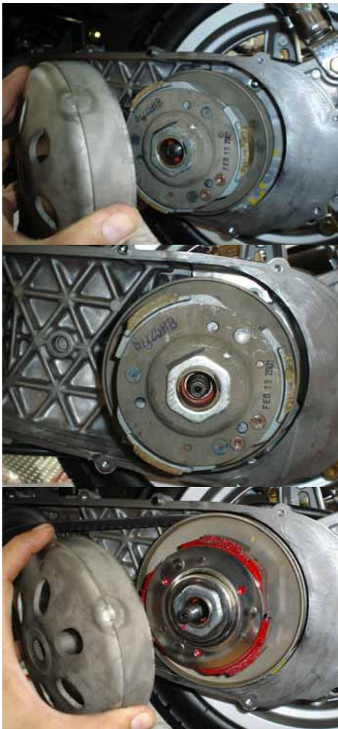
Next replace the stock clutch with the clutch from the power pack. If you do not have a race clutch you can always order one from MRP
