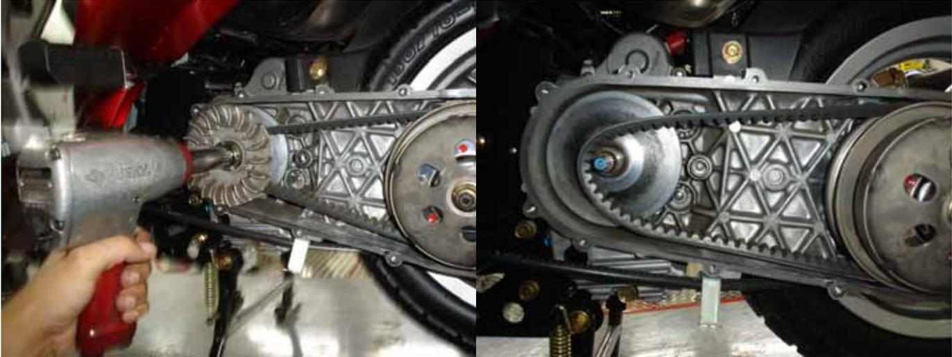
Step 4: With it removed slide the clutch bell off the input shaft. Now slide the complete clutch assembly off the input shaft. With the clutch securely held down, unscrew the nut that holds the clutch assembly together. Use extreme caution.
