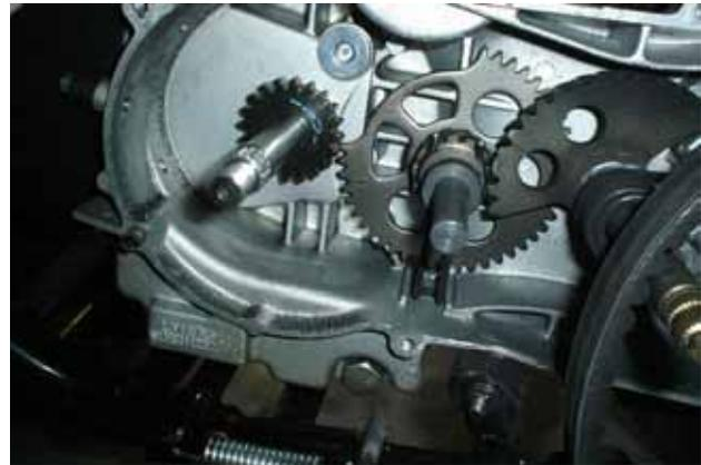
It should now look like this. (Notice there is no variator, spacer, or belt) Step 5: Replace with new Racing variator and spacer. Install new variator and spacer. After installing replace belt over variator. Once installed make sure to tighten everything before closing the cover.
