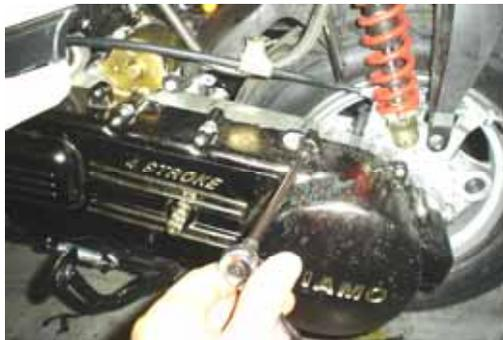
After replacing the cover make sure it looks like it originally did before the clutch replacement.
