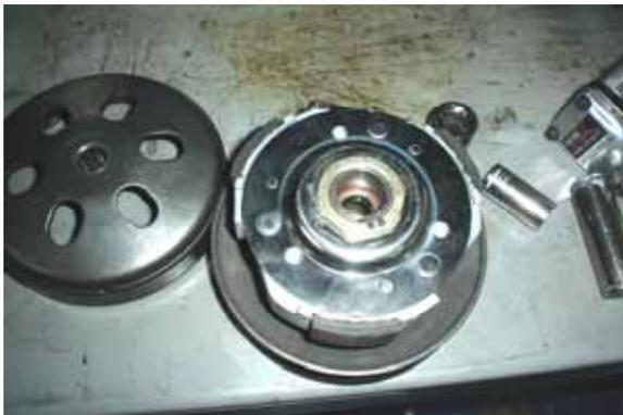
Identify Clutch – The clutch is in the rear and has a clutch bell cover.
