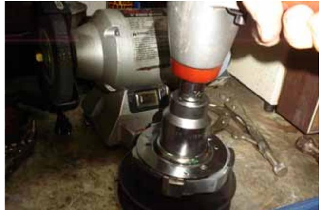
Step 2 Make sure to tighten with impact gun.
