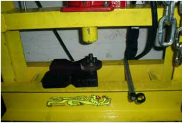
prepare to install the new MRP replacement 14 / 38 gear
