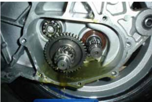
Then using a 10 to 20 ton press remove gently the gear
