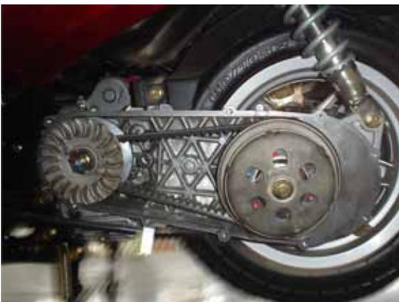
Step 2: Now that the transmission cover is off make sure to identify the parts we are changing. On the far left is the variator, in the center is the transmission belt, and on the far right is the clutch bell cover and the clutch
